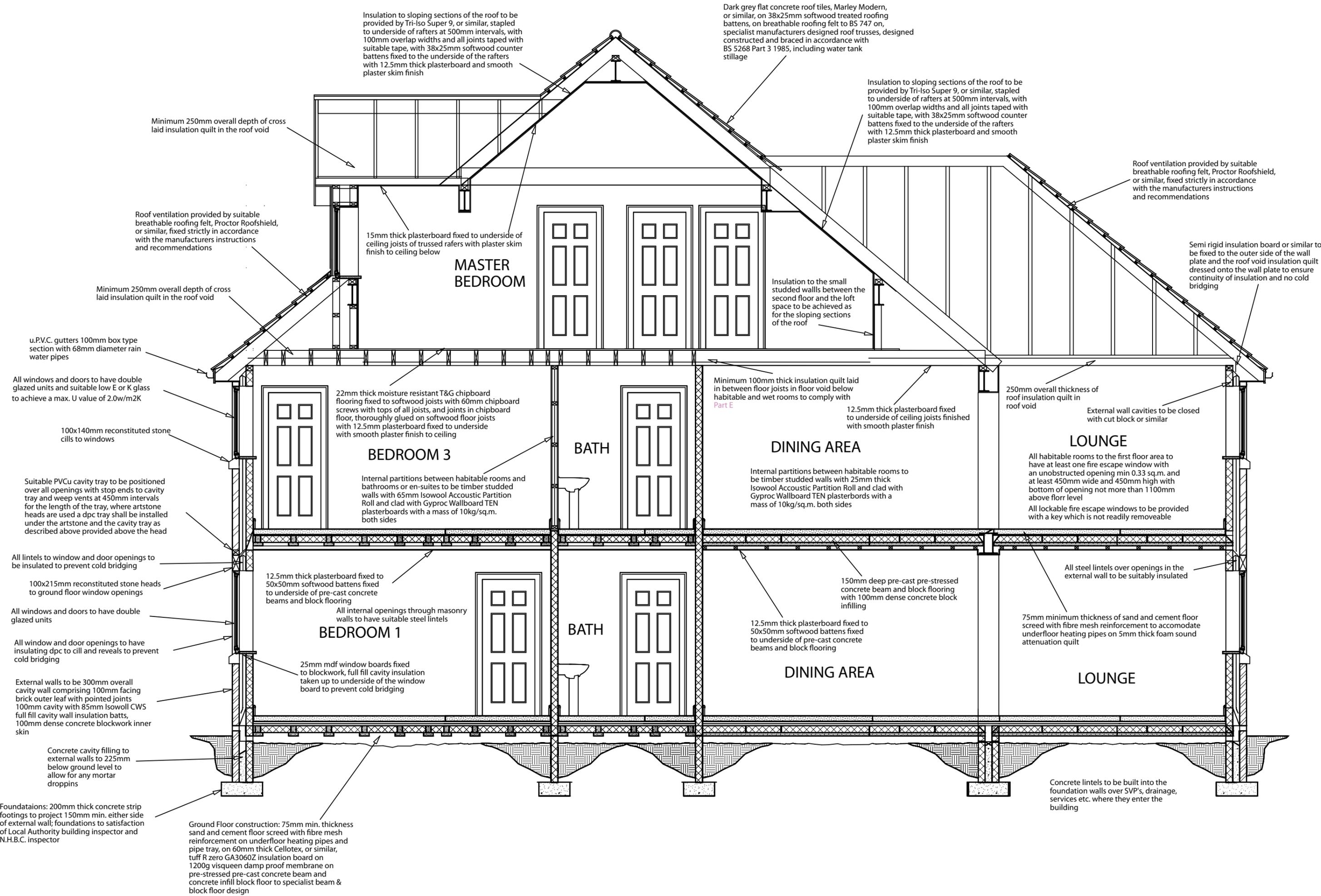
Insulation to sloping sections of the roof to be provided by Tri-Iso Super 9, or similar, stapled to underside of rafters at 500mm intervals, with 100mm overlap widths and all joints taped with suitable tape, with 38x25mm softwood counter battens fixed to the underside of the rafters with 12.5mm thick plasterboard and smooth plaster skim finish
